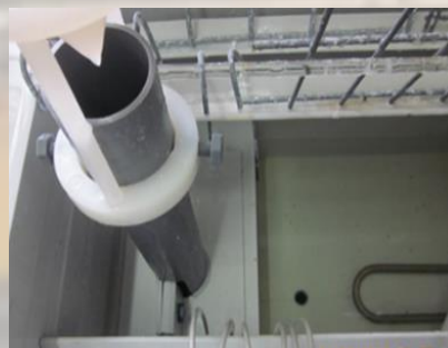
Salt Spray Test – according to BS Standard
