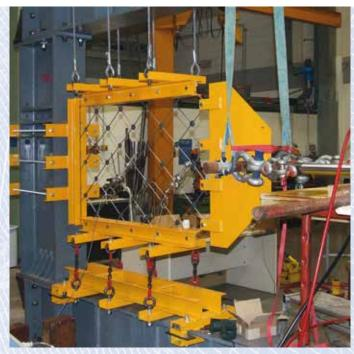
The ISOFIX covering has to give requisite support subject to differing angles of load .Tensile tests were carried out jointly with a National Research Institute to determine the load-bearing capacity in the vertical and horizontal direction.
